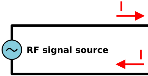
Figure ATL 2: Bifilar transmission line
