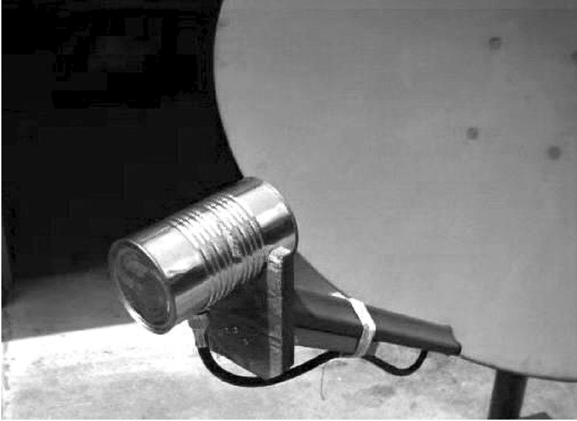
Figure ATL 13: Feed horn made from a food can.
