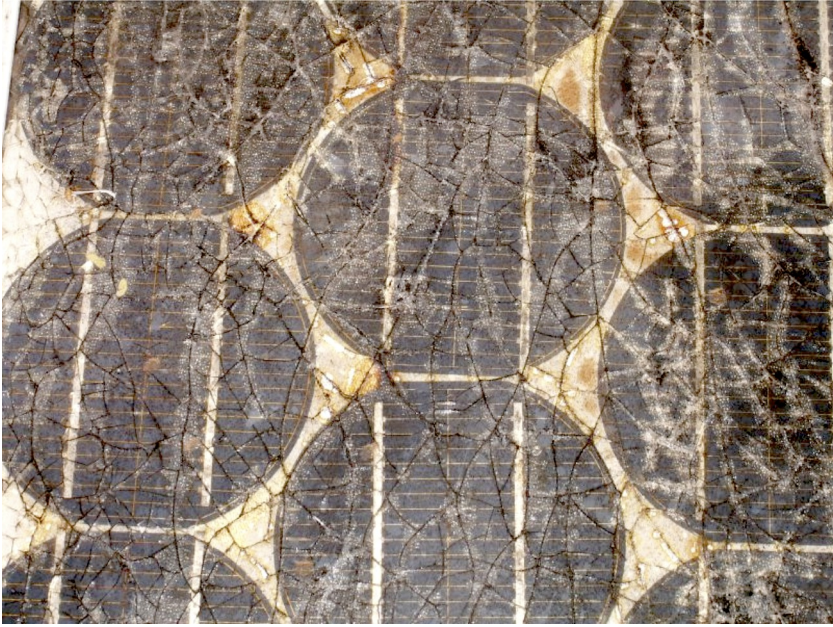
Figure OGP 6: The effect of water and corrosion in a solar panel
