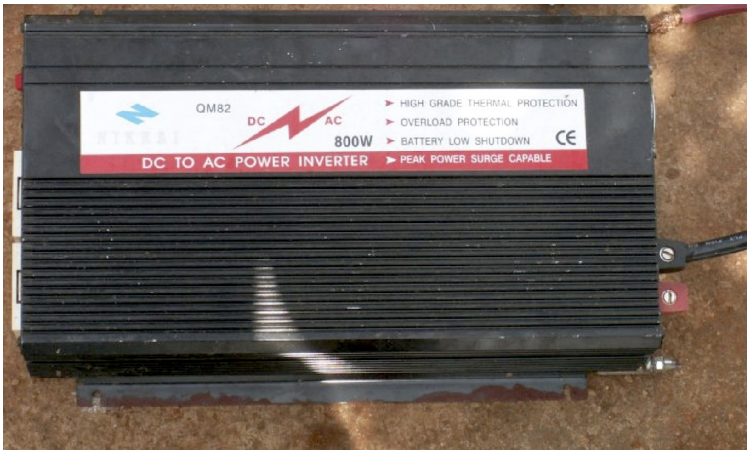
Figure OGP 4: An 800 Watt DC/AC converter (power inverter)
