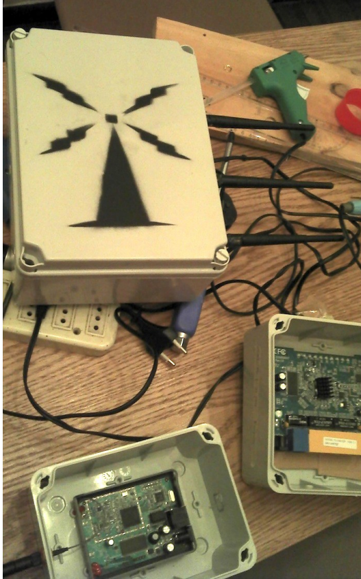
Figure MN 4:DIY outdoor routers based on PCBs taken from SOHO routers (Picture showing two devices based on TP-Link WR741 and WR941 and one based on a Fonera router)
