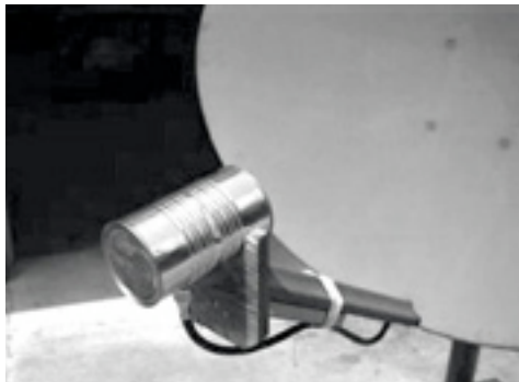
Figure 4.10: Feed horn made from a food can.
