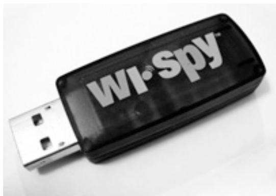
Figure 8.8: The Wi-Spy USB spectrum analyzer
